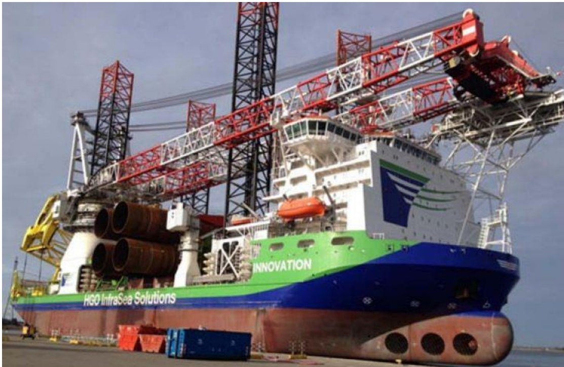
Figure 21: Innovation loaded with monopiles and transition pieces at Aalborg, Denmark for Westermost Rough wind farm, UK [42]
