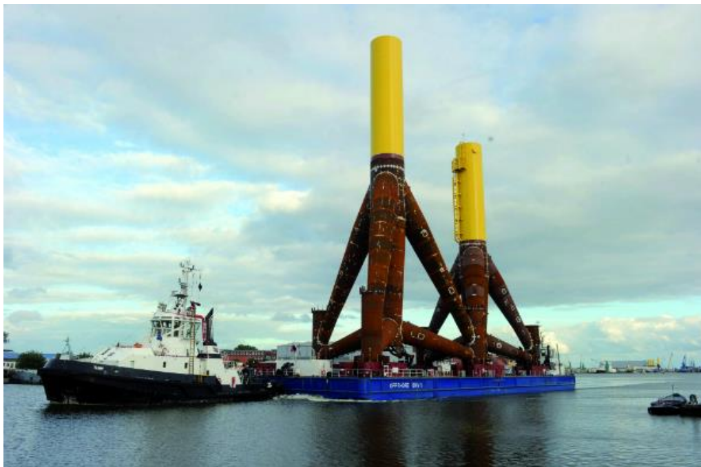
Figure 16: Two tripods are transported using BLG's OFFSHORE BHV 1 pontoon [35]
