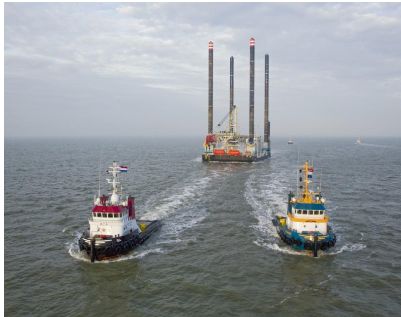
Figure 23: Self-Elevating Platform towed from Borwin Alpha site [44]
