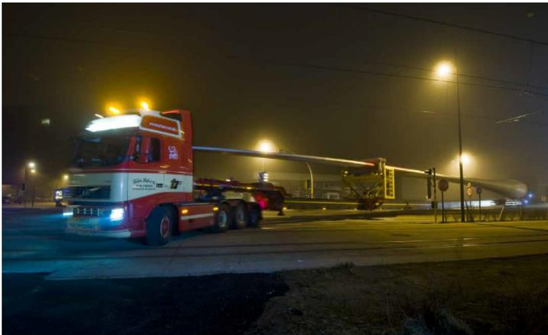
Figure 24: 63.5 m blade transported to the Port of Oostende [24]
