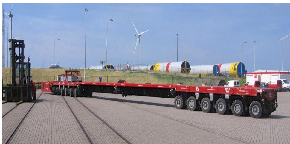
Figure 14: 2x6 axle line SPMT assembled as one self-propelled modular transporter (SPMT) [11]
